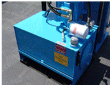
40 gallon oil reservoir
